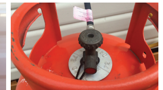
Turn the brass valve on top of each gas cylinder clockwise in the direction of 'close'.
